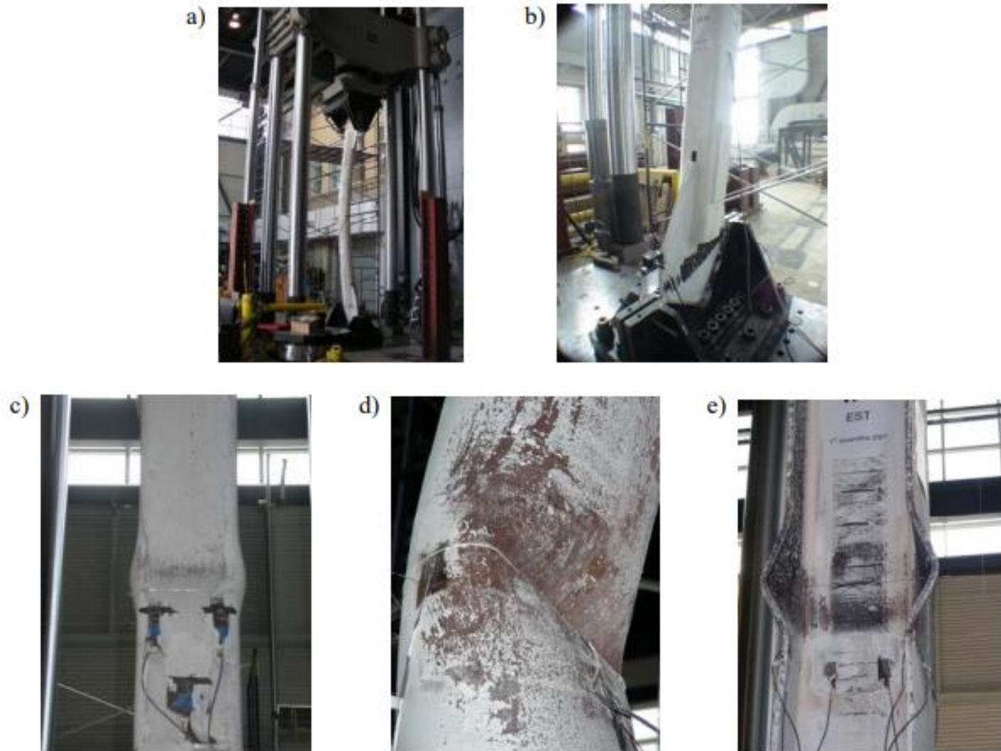
Figure 5 Observed brace behaviour: a) Overall buckling; b) Inelastic rotation in the gusset plate free length associated with buckling; c) Local buckling of a RHS brace specimen; d) Local buckling of a CHS brace specimen; and e) Local buckling of a W-shape brace specimen.
