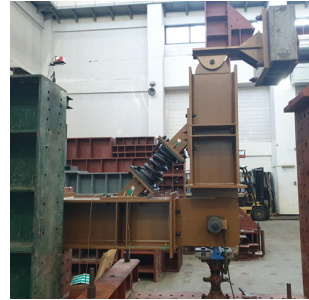
Fig. 4 Test setup for the seismic retrofit system subassembly
